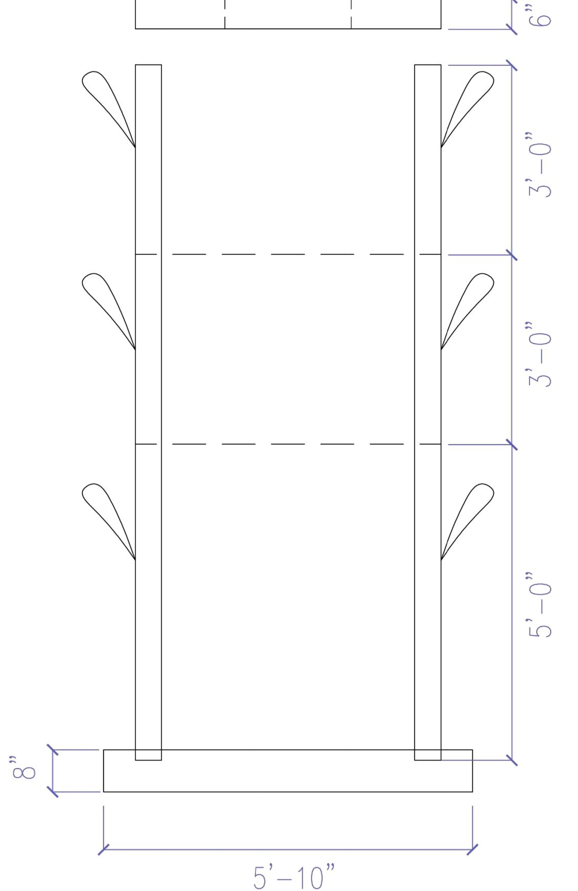
Lift Station made w/3500 PSI Concrete with  $6x6 \frac{6}{6}$  w.m.m. re—inforcement.
